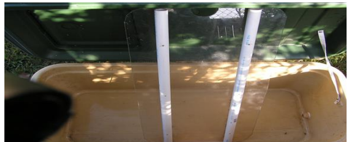
False bottom made by attaching 2 pieces of 3/4 inch PVC pipe to a plastic sheet. Custom fit to cooler bottom. Wood not recommended.
