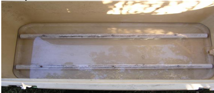
False bottom to prevent fish laying in blood, or water should you add addition ice.
